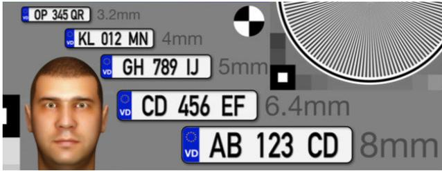
The next thing we included in the v.5.0 test chart is a variety of **licence plate** sizes positioned on the right hand side of the chart. We have reproduced plates that replicate those used in Europe (as well as other countries) with standard lettering sizes to cover
