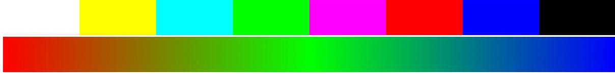
Both above and below the middle Siemens star you will find our traditional colour bars. Our software measures the **colour accuracy** of the eight television bars on top and shows them with their RGB values. This can be used for checking white balance accuracy of the system, together with the Macbeth colour chart. The continuous colour bar transitioning from red (on the left) to green (in the middle) and blue (on the
