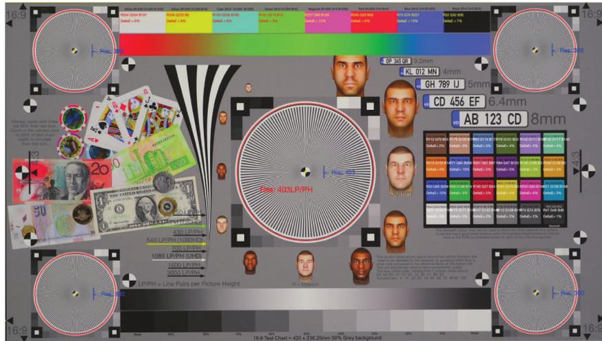
are proud to say that we have produced a very accurate sine-wave Siemens stars. Our stars consist of 144 rays, displaced at 2.5° each, and printed in high quality on our latest test chart, granting accurate measurements of resolution.
