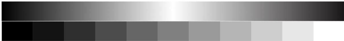
With our software, the observer can now evaluate the continuity and shape of the black-white-black bar at the bottom, and produce the luminance change curve, which reveals the **image processing qualities** of the camera. The observer can also check the luminance of the 11 grey steps at the bottom, and display a graph of the luminance change, which
